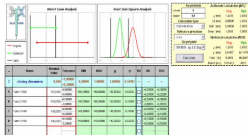
Figure 9. Tolerance chain analysis tool in DFX Platform
